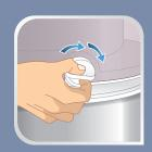
• Screw back and tighten up the boiler rinse cap.
