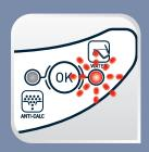
The red «Water tank empty» button light is flashing: the water tank is empty. See paragraph «Refilling the water tank during use»
