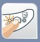
The next time you use the generator hold down the "OK" button for a few seconds to turn off the orange light.
