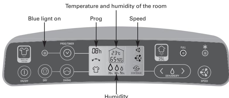
With your appliance switched off, press the "PROG/TIMER" key (F) as many times as necessary to define the number of hours before automatic start-up.
