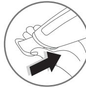
For liquids on smooth surfaces, insert the squeegee attachment for liquids\* in the suction inlet.
