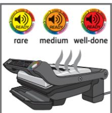
**11** According to the degree of cooking, the indicator light changes colour. When the indicator light is yellow with a beep, your food is rare, when the indicator light is orange with a beep, your food is medium and when the indicator light is red, your food is well done.
